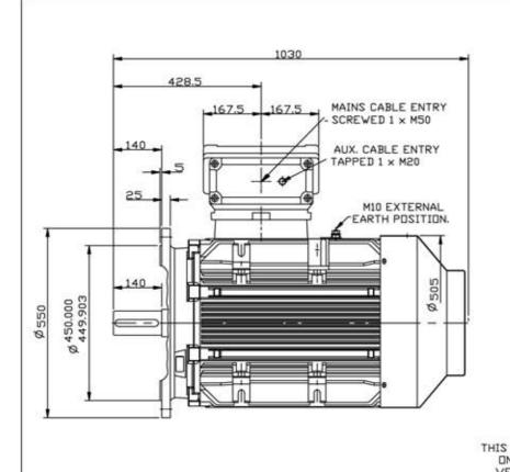
220 2 LIFTING LUGS DIAGONALLY OPPOSITE. 8 HOLES Ø19 THIS LIFTING LUG FITTED EQUALLY SPACED ONLY WHEN MOTOR IS ON 500 P.C.D. VERTICALLY MOUNTED.
